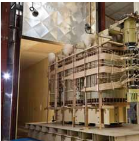
• Vapor phase drying up to 1000MVA
