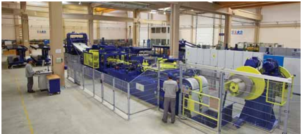
• 1000mm GEORG length core cutting machine
