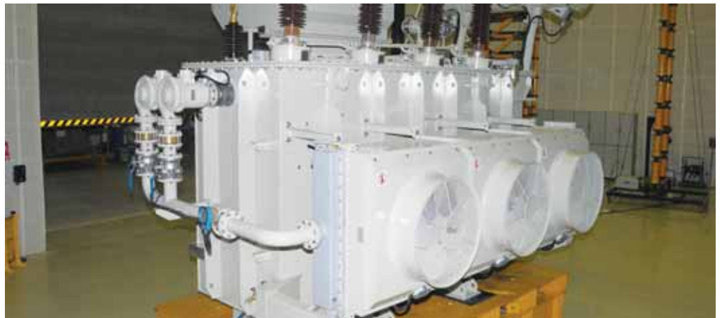
• Transformer with OFWF cooling
