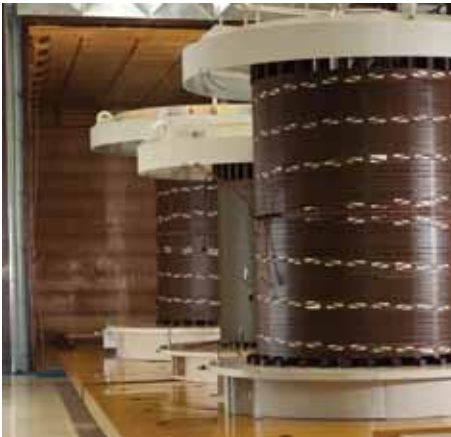
• Winding drying oven (Dynamic pressing)
